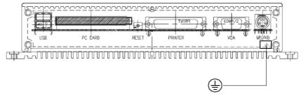
Figure 3.1: Chassis Grounding Connection
